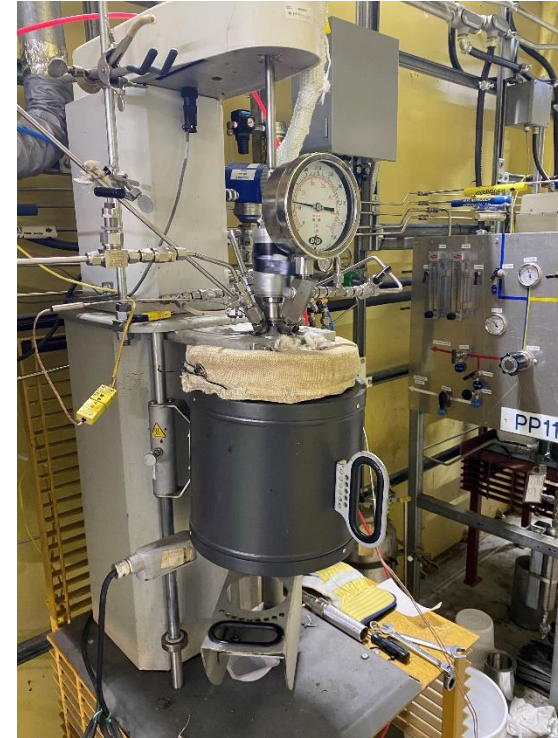
250 mL batch reactor unit for catalyst evaluation studies
