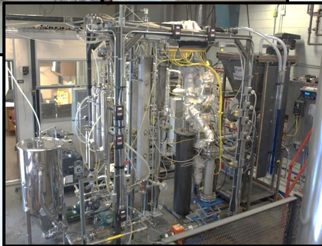
Screw reactor (above), Fluid Bed Fast Pyrolysis (right)
